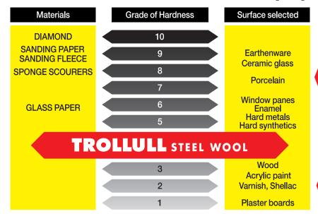
These robust surfaces can be cleaned and processed scratch-free with steel wool
